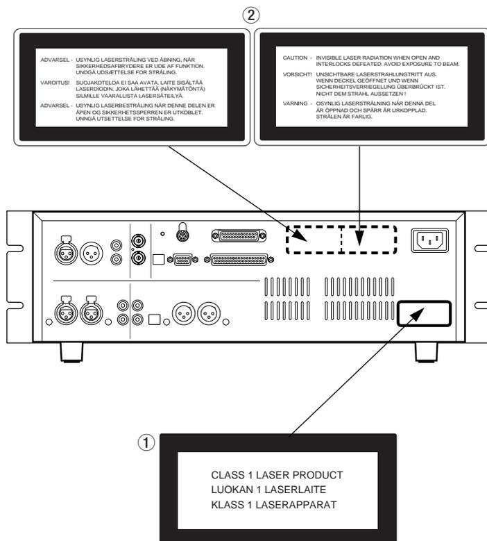
① THIS LABEL IS ATTACHED TO THE PLACE AS ILLUSTRATED TO INFORM THAT THE APPARATUS CONTAINS A LASER COMPONENT.
